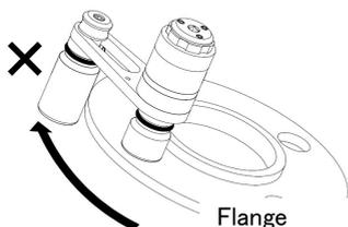
※ Do not receive output torque by outside of socket on the square shank or Flange etc.
