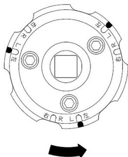
When rotate the output angle adjustor to the right, set the clutch dial to the Right (R)
