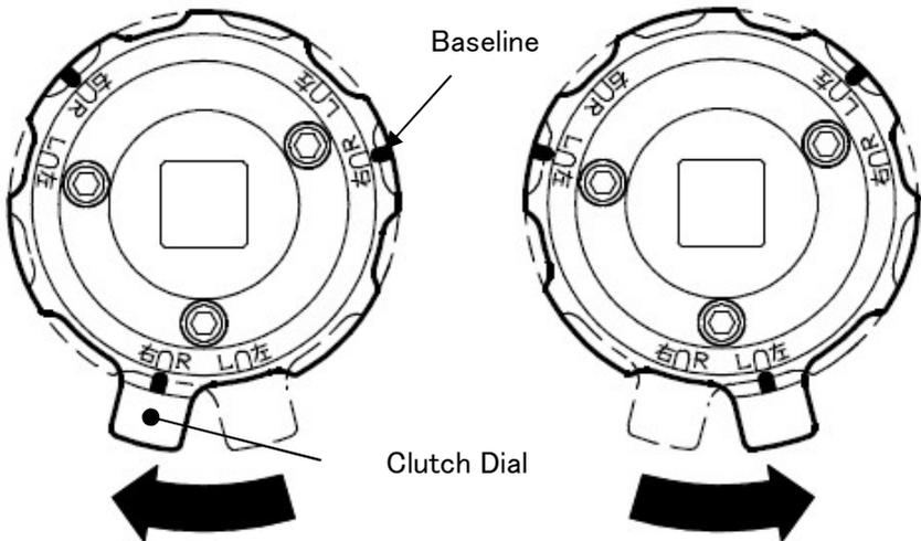
When rotate clockwise, adjust the baseline to Right (R).
