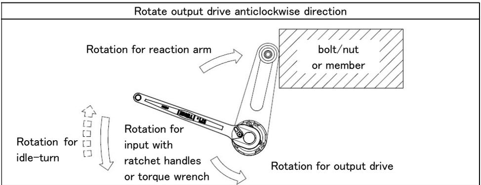
**Note** In case of using torque wrench, when reaching preset torque, the wrench makes a clicking sound as well as a light retroaction.
