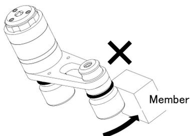
※ Do not place drive square or outside of socket against a solid member or surface adjacent to the bolt/nut to be tightened or loosened, as such member or surface receives large force almost equivalent to output torque.
